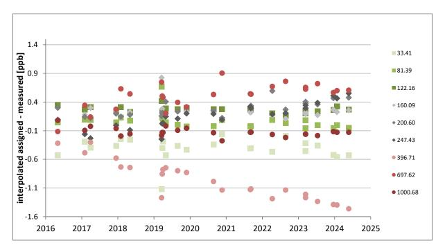
Figure 23 Time series of quadratic regression fit residuals of LGR CO calibrations for FCL Primary Standards
