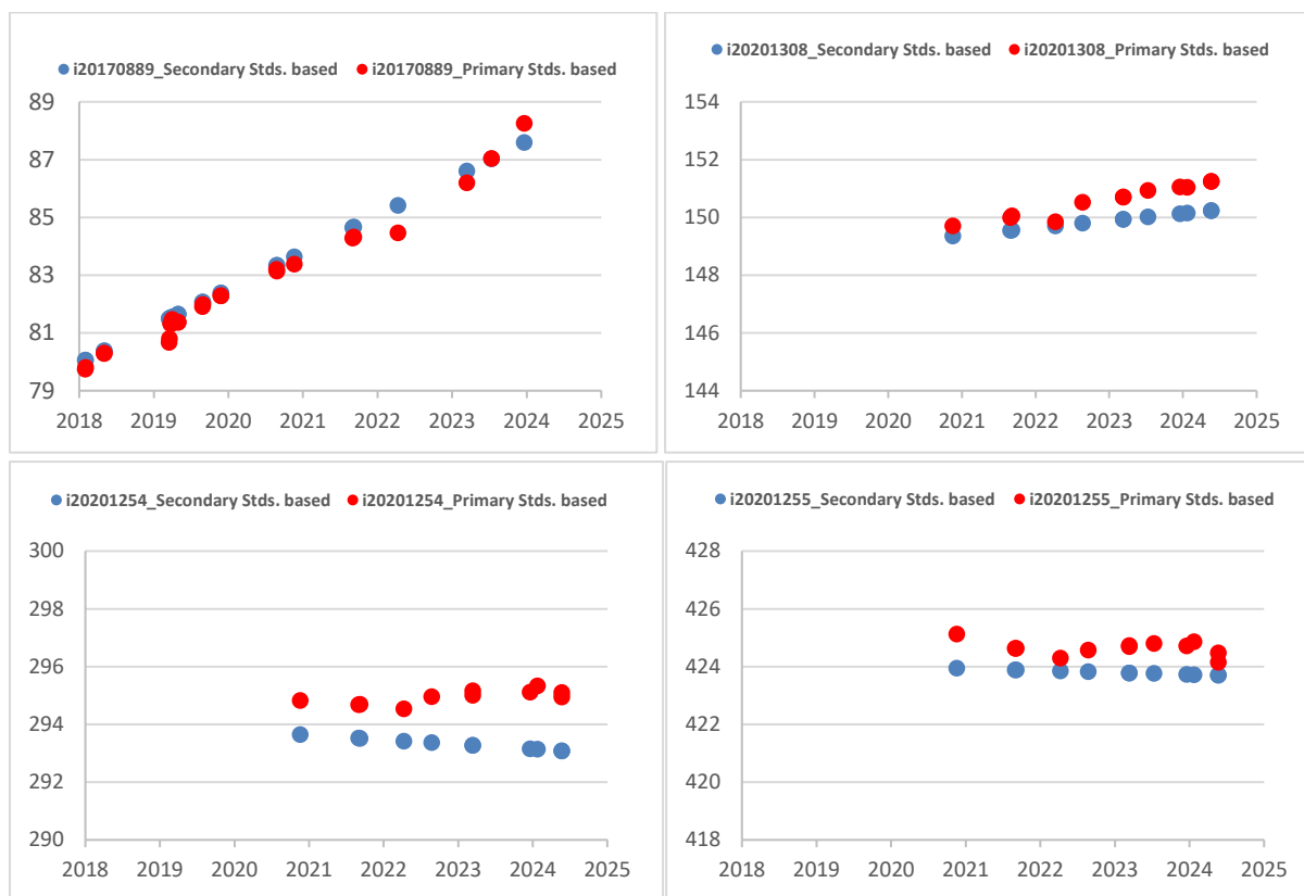
FIGURE 24: SECOND SET OF SECONDARY CO STANDARDS: ASSIGNMENT RECORD AGAINST FCL'S PRIMARIES (RED DOTS) AND CO MOLE FRACTIONS BASED ON ASSIGNED TREND FUNCTIONS RELATING TO FCL'S FIRST SET OF SECONDARIES (BLUE DOTS) (VALUES IN [PPB]).
