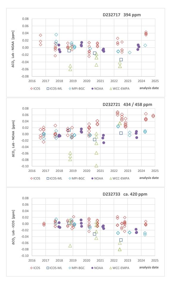
Figure 11 CO<sub>2</sub> offset in MENI ICP between FCL, MPI, ICOS MobileLab and WCC relative to NOAA
