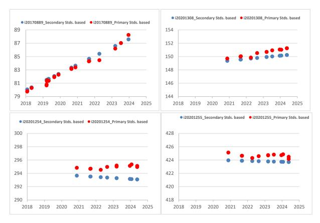
Figure 25 Second set of Secondary CO Standards: assignment record against FCLI's Primaries (red dots) and CO mole fractions based on assigned trend functions relating to FCL's first set of Secondaries (blue dots) (values in [ppb]).
