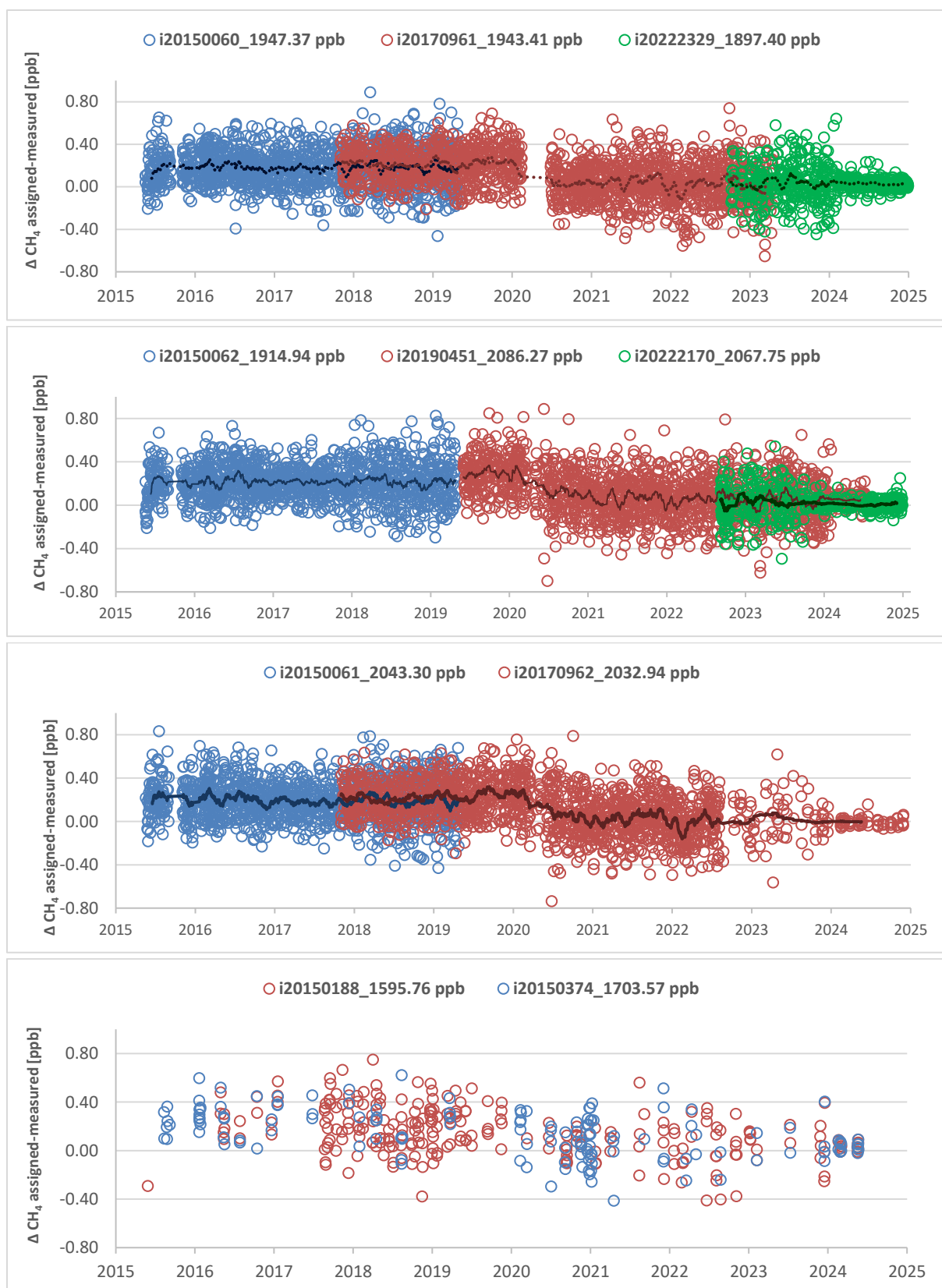
FIGURE 13: TIME SERIES OF THE \text{CH}_4 OFFSET OF TARGET MEASUREMENTS TO THEIR RESPECTIVE ASSIGNED VALUES. The dark line represents a 30 points-running mean.
