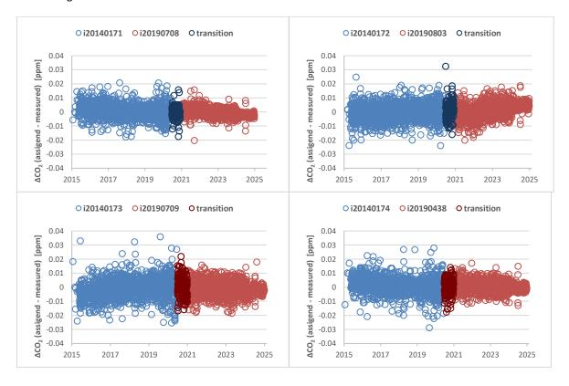
Figure 4 Time Series of CO<sub>2</sub> linear regression fit residuals of the FCL Sencondary Standards. Blue symbols represent the first set of FCL Secondary Standards, red symbols the second set of FCL Secondary Standards. The dark symbols are indicating the transition phase when onlytho of the standards were replaced
