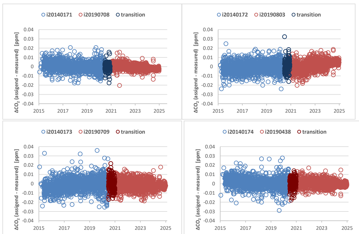
FIGURE 3: TIME SERIES OF CO 2 LINEAR REGRESSION FIT RESIDUALS OF THE FCL SECONDARY STANDARDS. Blue symbols represent the first set of FCL Secondary Standards, red symbols the second set of FCL Secondary Standards. The dark symbols are indicating the transition phase when only two of the standards were replaced.
