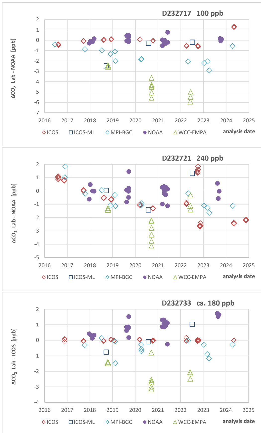
FIGURE 31: CO OFFSET IN MENI ICP BETWEEN FCL, MPI, ICOS ML AND EMPA RELATIVE TO NOAA (LOWEST PLOT: RELATED TO ICOS)
