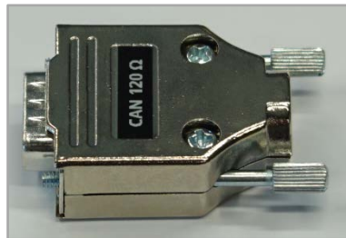
Figure 15: CAN terminating resistor (120 Ω)
