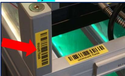
8. Assign each inserted flask to a port check for the confirmation blink signal at the drawer (first scan the port-barcode and secondly scan the barcode on the flask):
