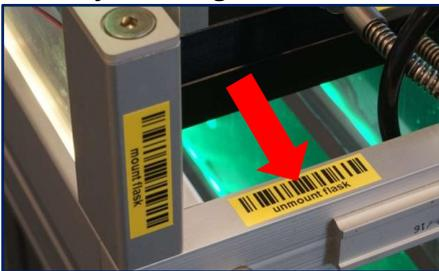
3. Scan the flasks to be removed and check for the green confirmation blink signal at the drawer (use either clamp barcode or the flask barcode, it doesn't matter) and check if all flasks have been scanned.
